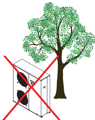
Figure 6.8: incorrect installation of the external unit.
